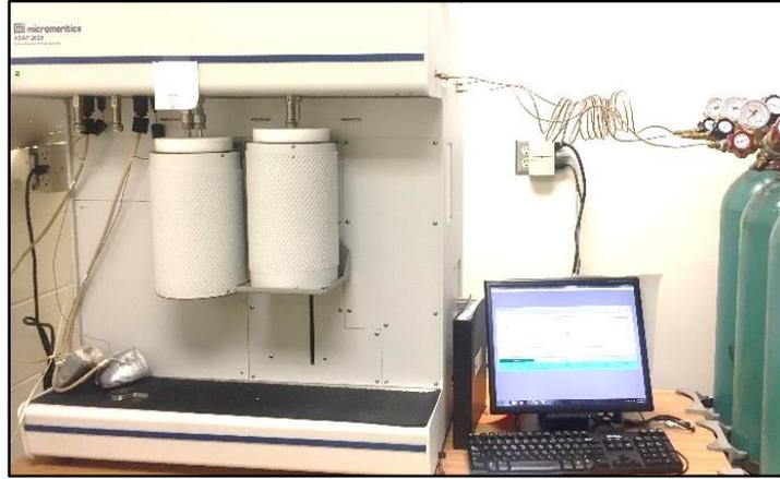
*Figure 3-5 Specific surface analyzer (ASAP 2020 Micromeritics)*
