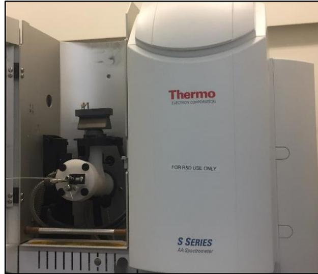
Figure 3-6 Atomic absorption spectrometer
