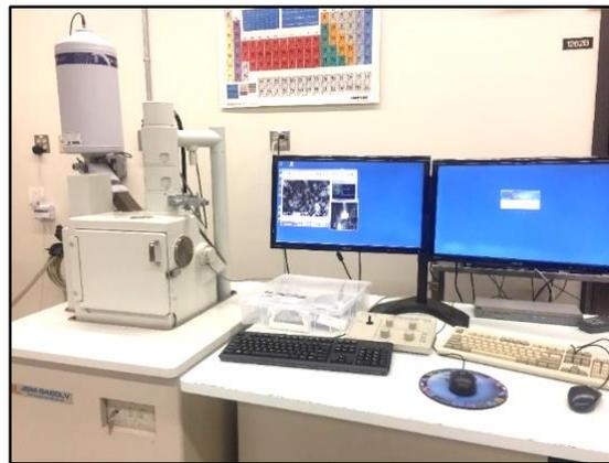
*Figure 3-4 SEM-EDX instrument (JEOL JSM-6460)*
